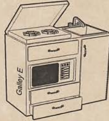
GALLEY E Space for *microwave, or use space for storage with a door. Stove and propane system can be deleted for credit. Sink/Stove can be switched.
