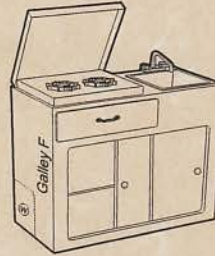
GALLEY F 18" allows walk space when located across from gauchio bed. Sliding or hinged doors, same cost. Sink/Stove can be switched.
