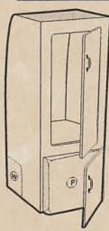
CLOSET B Clothes hanging height is 32". Shelf over bottom compartment hinges up for hanging height of 47"
